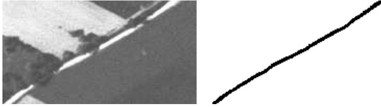
FIGURE 18. An aerial image (© IGN) with occlusions and the result of applying E = E_0 + E_{\text{gap}} to this image. Parameter values: [\lambda = 1, \alpha = 0.14, \beta = 0.06, \lambda_i = 2.9, \alpha_i = 0.3, \beta_i = 2.9, \beta_A = 6] .
