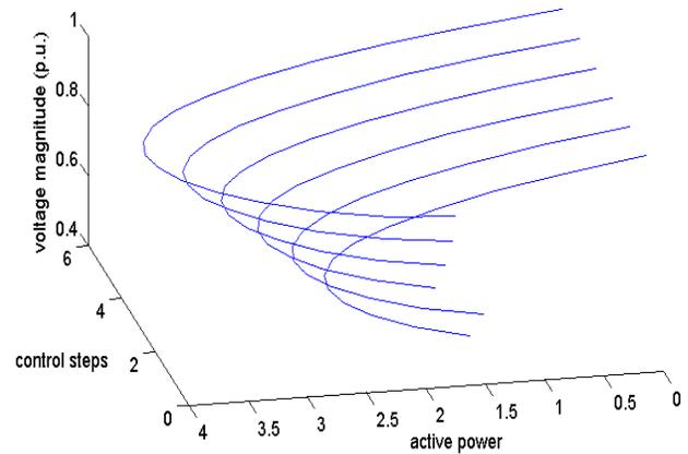
Fig. 5. loadability enhancement with different control steps
