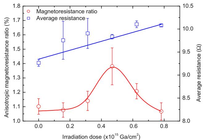
**Figure 5.** Anisotropic magnetoresistance ratio and baseline resistance of 20 nm NiFe/2.5 nm Au bilayers as a function of  $\text{Ga}^+$  irradiation dose. The solid lines represent a linear fit to the average resistance data and a guide to the eye for the AMR data.
