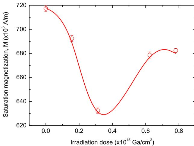
**Figure 3.** Variation of  $M_s$  with dose for  $1.3 \times 5.5$  mm 20 nm NiFe/2.5 nm Au samples measured using SQUID magnetometry which show a drop followed by a recovery in the magnetic moment. The line is a guide to the eye.
