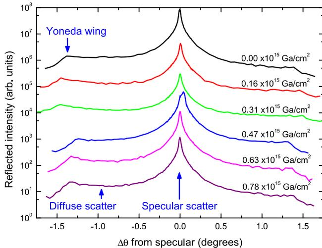
**Figure 7.** Rocking curves ( $\Delta\theta$ ) recorded at a Keissig maximum as a function of  $\text{Ga}^+$  dose. The specular scatter is located at  $\theta = 0$  with the critical angles marked by the Yoneda wings which are symmetrically positioned either side of the specular ridge. Curves are offset for clarity.
