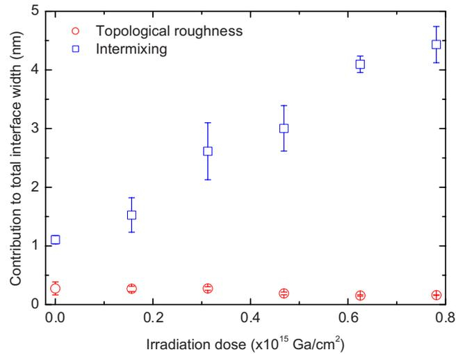
**Figure 8.** Differentiation between roughness and intermixing contributions to the interface width shows a constant roughness contribution and an increasing interface width that is accounted for by an increase in the chemical intermixing.
