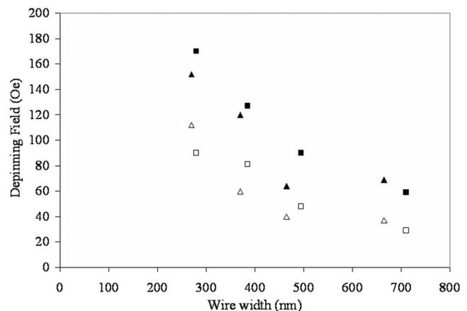
FIG. 4. Injection fields (open symbols) and notch depinning data (solid symbols) for ( $\blacksquare$ ) rectangular notches and ( $\blacktriangle$ ) triangular notches respectively measured by MOKE. All notches have a nominal depth half that of the wire width.
