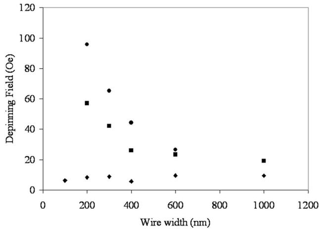
FIG. 2. Switching field as a function of wire width of a 5 nm thick Permalloy nanowire. ( $\blacklozenge$ ) represents magnetization reversal of the nucleation pad, ( $\blacksquare$ ) represents domain wall injection from the nucleation pad into the wire, and ( $\bullet$ ) represents domain wall depinning from a triangular notch patterned along one side of the nanowire.
