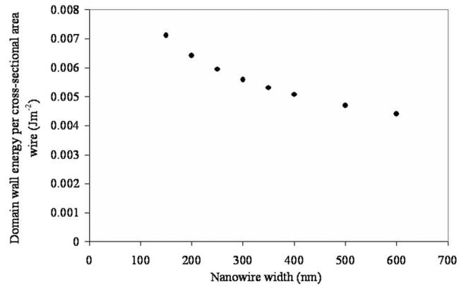
FIG. 3. Plot of domain wall energy per unit cross-sectional area as a function of nanowire width, deduced from OOMMF micromagnetic simulations.<sup>8</sup>
