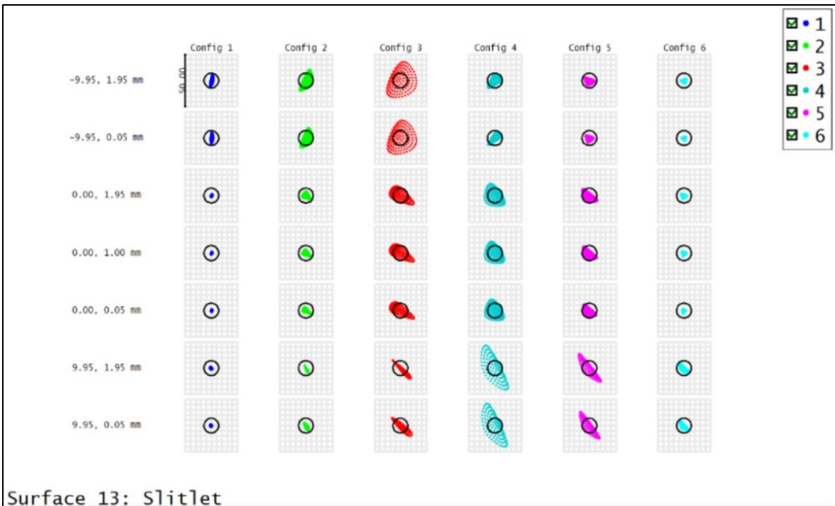
Figure 2. Optical quality obtained for the HR (top) and LR (bottom) image slicers. Each column represents a slitlet defined by seven field points. The circle is the Airy disk, showing the diffraction limit. Configurations 3 and 4 corresponds to the slices with the largest off-axis distances.
